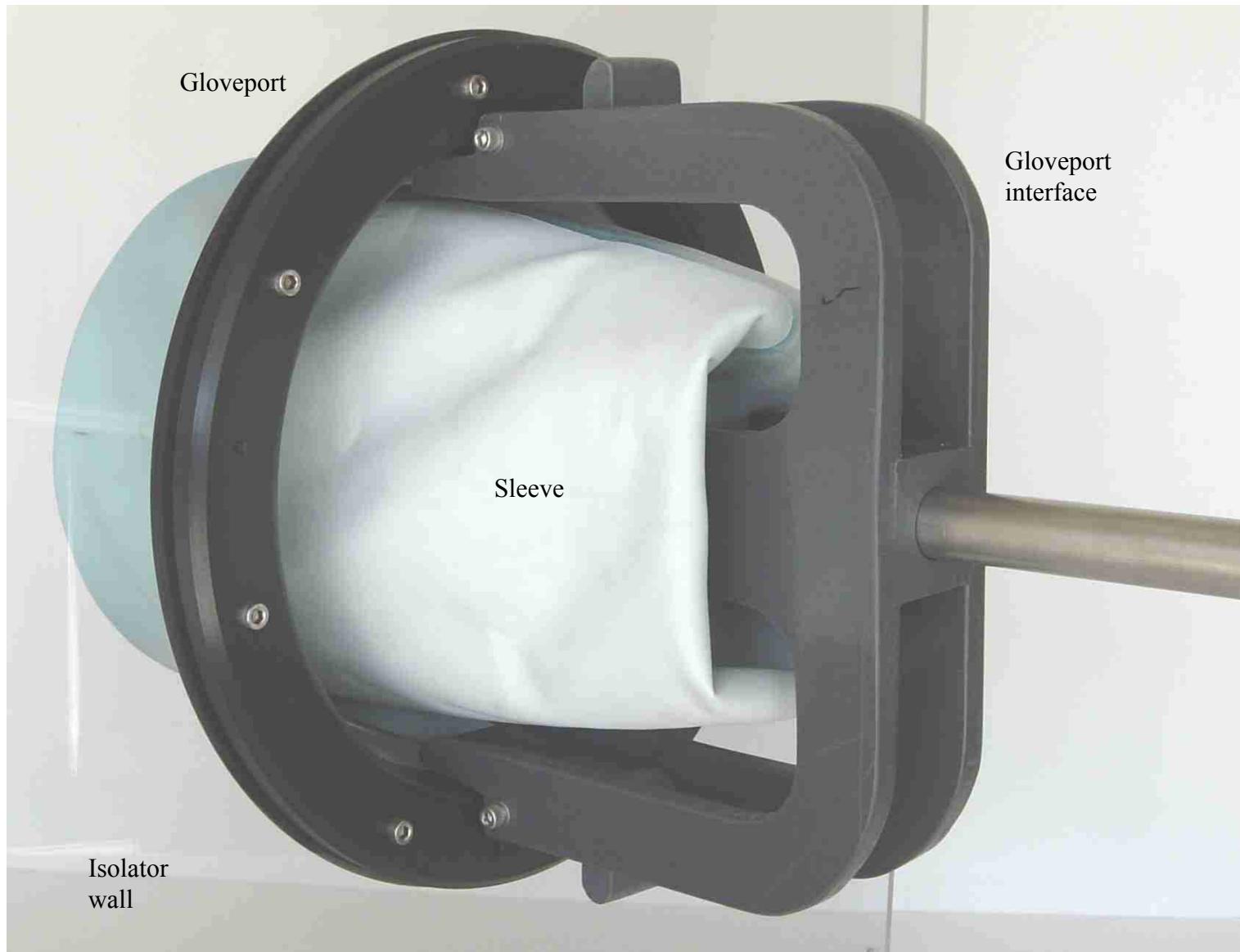
Sleeve geometry - as seen from outside the isolator
